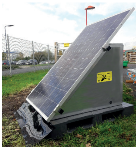
Figure 3.1: PVC strip prevents shadows on the solar panel caused by grass growth
